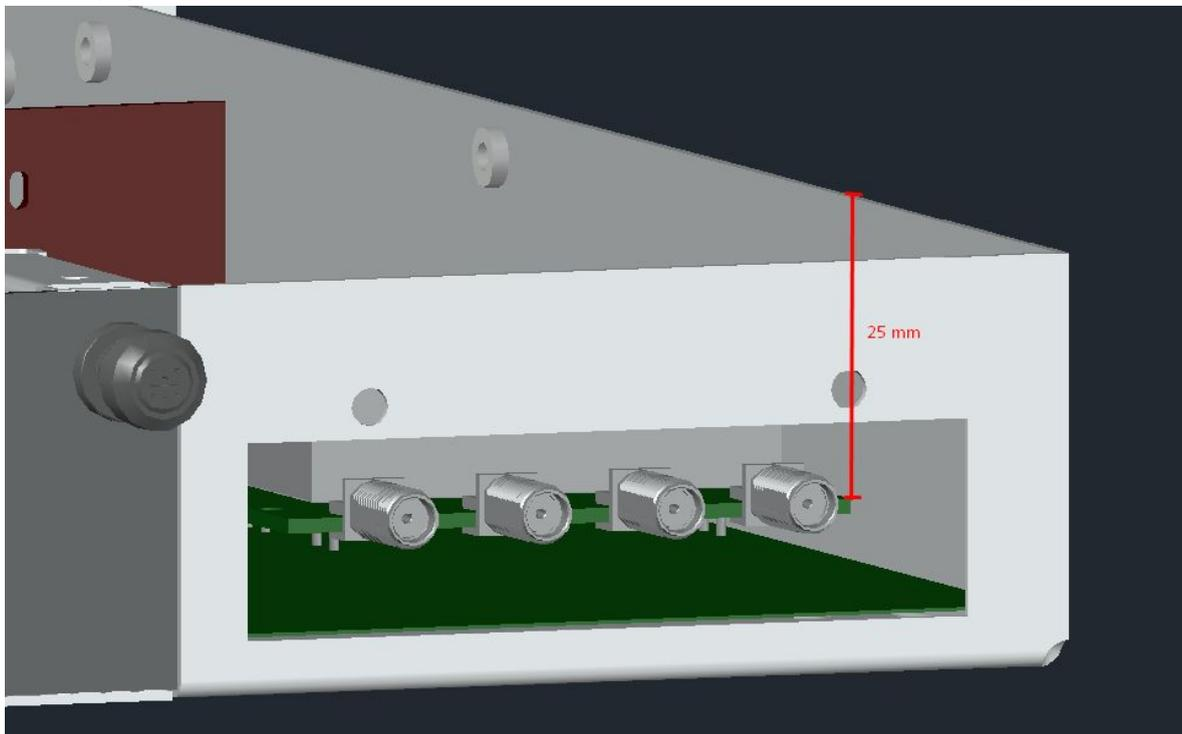
Figure 8: Height available from the top of a FMC board.
