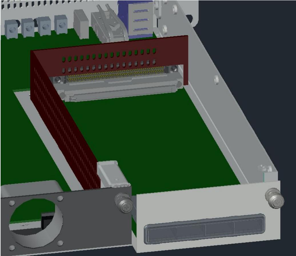
Figure 5: Expansion board with 4 QSFP ports.
