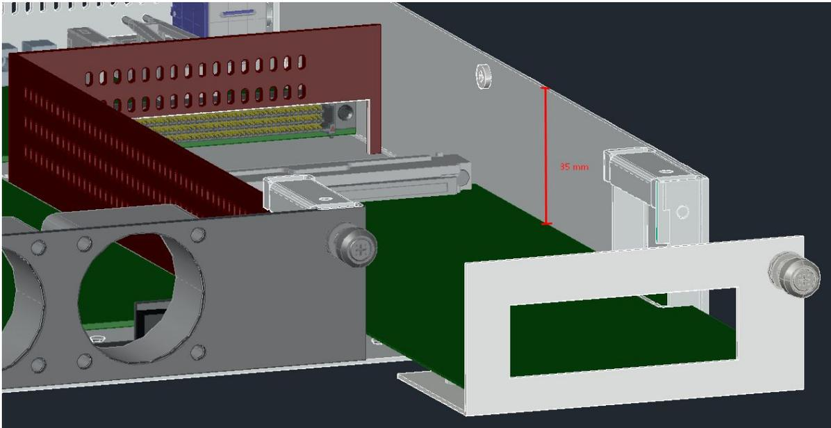
Figure 9: Height available from the expansion board with tray.
