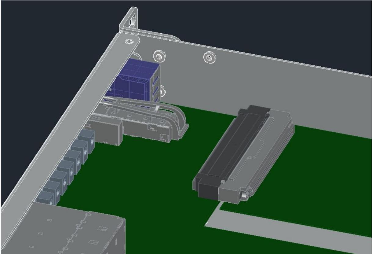
Figure 6: SEAF-SEAM connectors.
