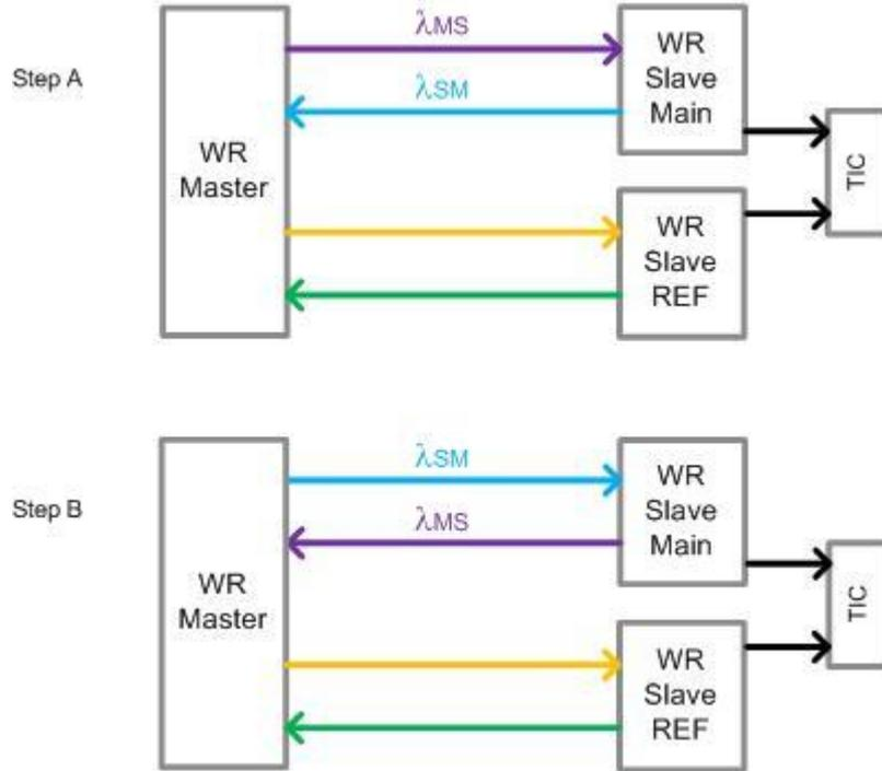
**Figure 8.** Calibration principle with WR reference link as replica of the WR Master 1PPS
