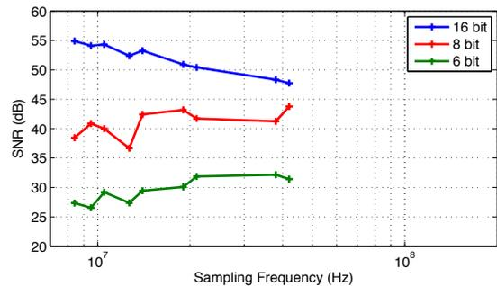
Fig. 10. SNR vs CORDIC Resolution for the (IF = 2 MHz)
