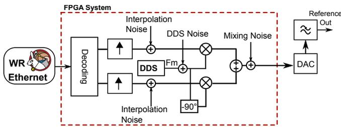
Fig. 4. System Architecture of the Slave Node
