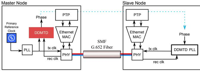
Fig. 1. WR Network System Architecture
