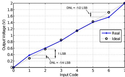
Fig. 6. DAC Differential Nonlinearity Errors
