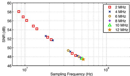
Fig. 8. SNR vs ADC Sampling rates that down-convert for the input signal to several IF
