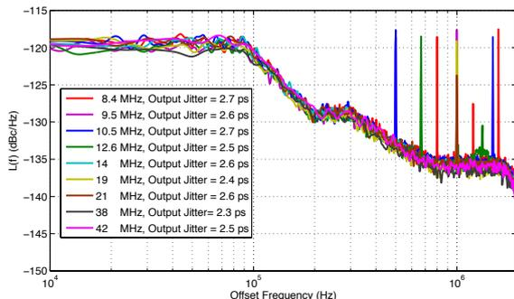
Fig. 12. Phase-Noise Spectrum for different sampling rates (IF = 2 MHz)
