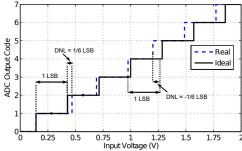
Fig. 5. ADC Differential Nonlinearity Errors
