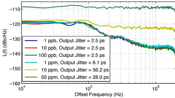
Fig. 11. Phase Noise spectra of the output waveform for different rms jitter in the slave's frequency reference
