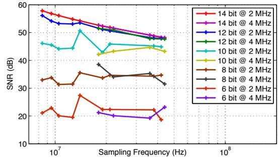
Fig. 9. SNR vs Number bits of the ADC for different IF signals (IF = [2, 4] MHz)
