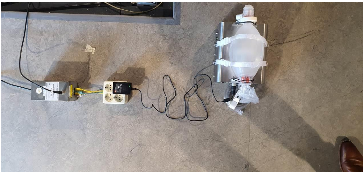
Figure 6: Conducted immunity set-up. The insulated floor is 10cm above the ground plane.
