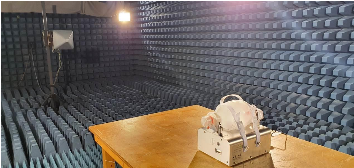
Figure 2: Photo showing the VentilatorPAL in the FAR (the mobile telephone is not visible).
