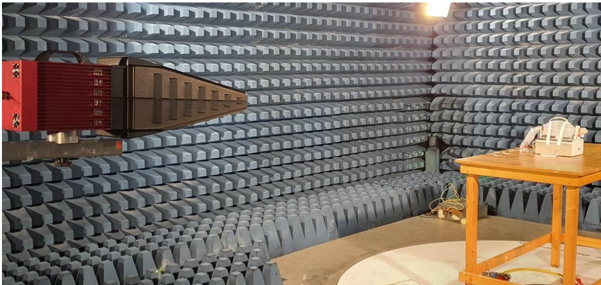
Figure 3: Photo showing the VentilatorPAL test set-up
