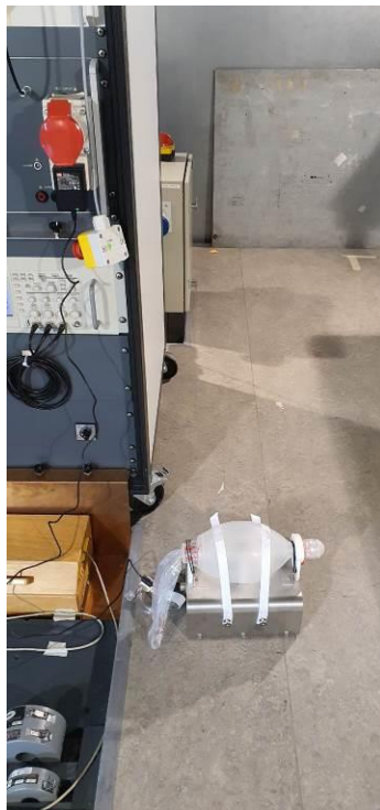
Figure 7: EFT immunity set-up. The insulated floor is 10cm above the ground plane
