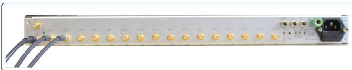
Figure 11: Pulse Distributor with “IN B”, “OUT 1” and “OUT 2” connections
