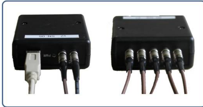
Figure 12: USB-interconnection-box front (USB, 2xLEMO) and back side (5xLEMO)
