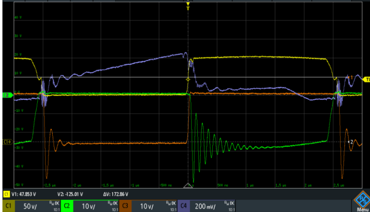
Fig. 6: C_{sn} = 220pF (for forward diode, shown in green above).
