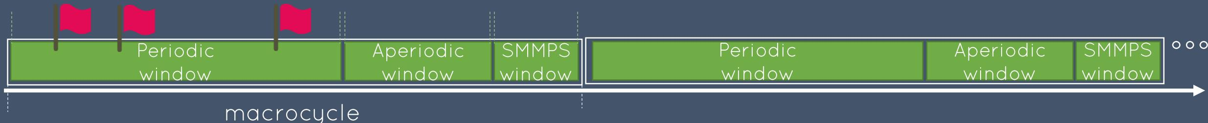
The macrocycle (length of each window and variables in periodic window) is configured once at startup and is not changed during bus operation.
