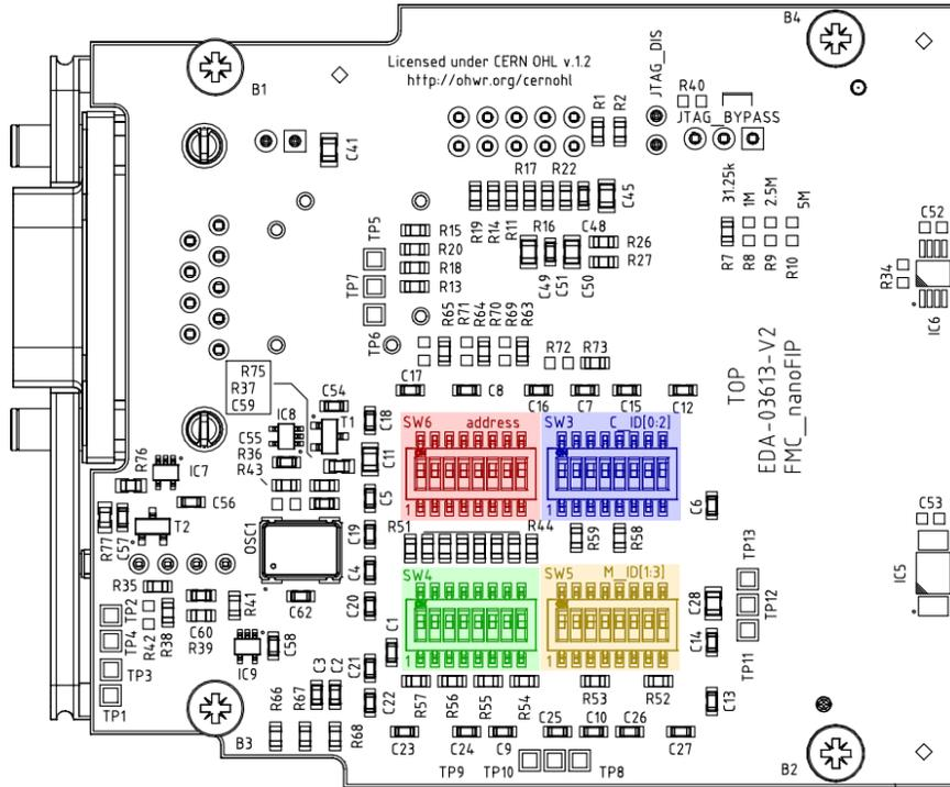
Figure 3: Configuration DIP switches.
