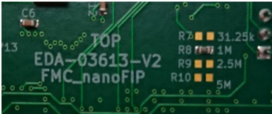
Figure 2: Resistors indicating the board variant.
