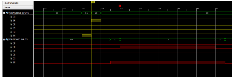
Figure 5.2: Input pulses (yellow) and corresponding stretched signals (red). Input 0 is stretched by 10 cycles, input 4 by 8, hence the difference in pulse widths.
