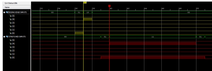
Figure 5.1: Input pulses (yellow) and corresponding stretched signals (red). Input 0 is stretched by 10 cycles, input 4 by 8, hence the difference in pulse widths.
