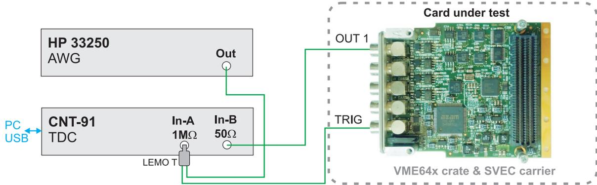
Figure 1: Long term measurement setup.
