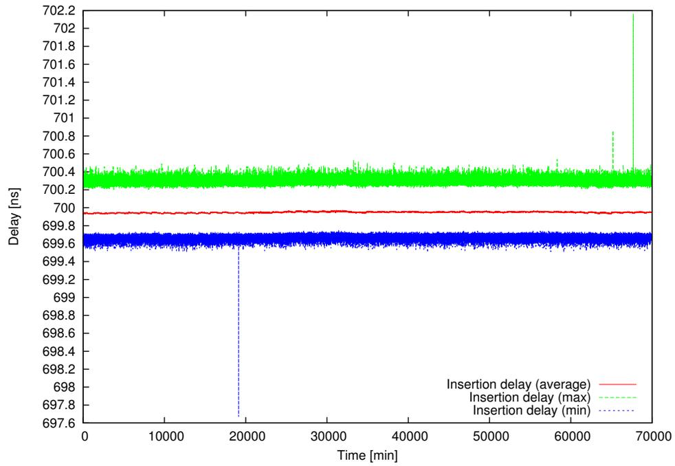
Figure 2: Average, minimum and maximum trigger-to-output delay (sliding average with a 1-minute window).
