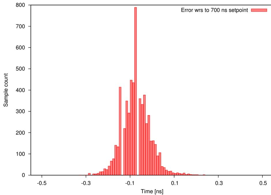
Figure 3: Histogram of trigger-to-output jitter.
