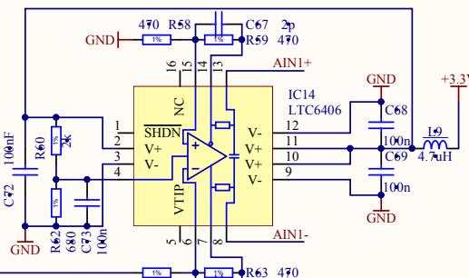
resistor divider creates potential of 0.9V for VOCM inputs (common mode output potential)
