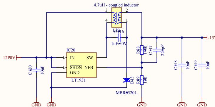
△ CUK inverting DC/DC converter. According to the datasheet - output ripple: 1mV.
