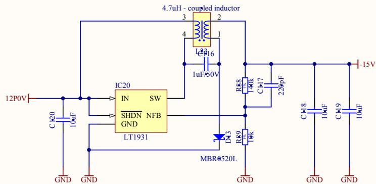
CUK inverting DC/DC converter. According the datasheet - output ripple: 1mV.
