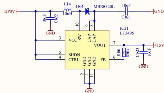
standard low noise boost converter. According to the datasheet, output ripple approx. 10mV
