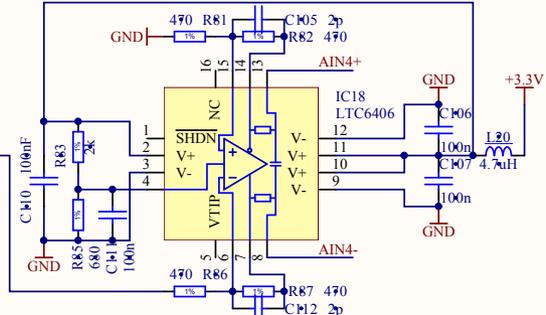
resistor divider creates potential of 0.9V for V<sub>OCM</sub> inputs (common mode output potential)
