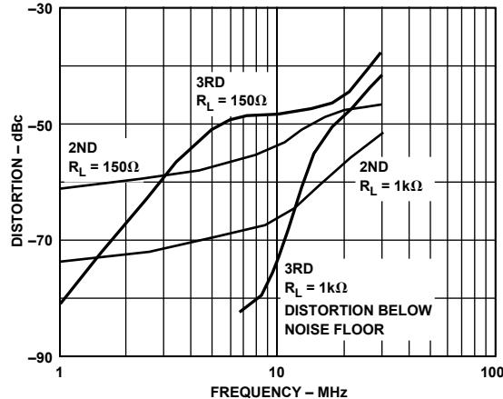
Figure 15. Distortion vs. Frequency;  $V_S = \pm 5$  V,  $G = +2$
