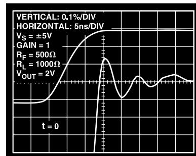
Figure 18. Settling Time
