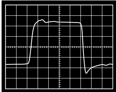
Figure 19. Large Signal Step Response;  $V_S = \pm 5 V$ ,  $V_O = 4 V$  Step
