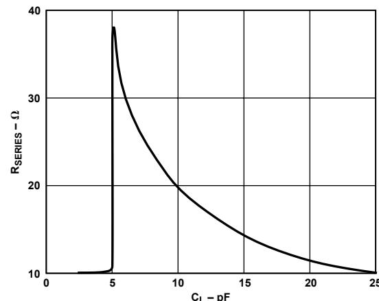
Figure 26. Driving Capacitive Load
