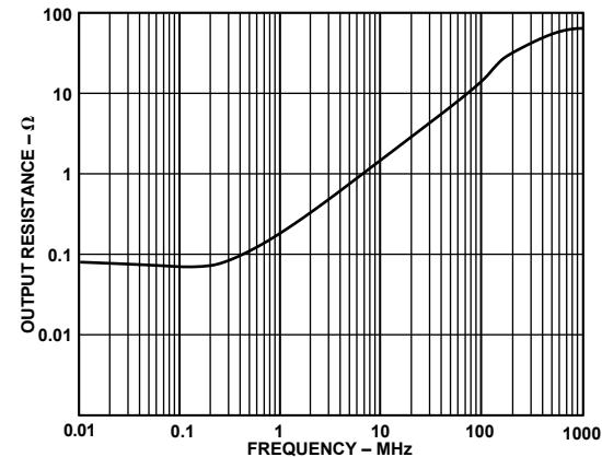
Figure 17. Output Resistance vs. Frequency,  $V_S = \pm 5$  V and +5 V
