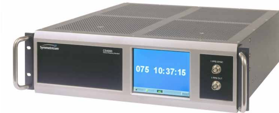
Figure 1 Cs4000 Front Panel w. Optional LCD Touchscreen (DCC Option)
