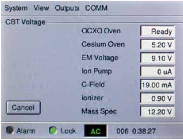
Figure 41 CBT Supplies (CBT Voltage)
