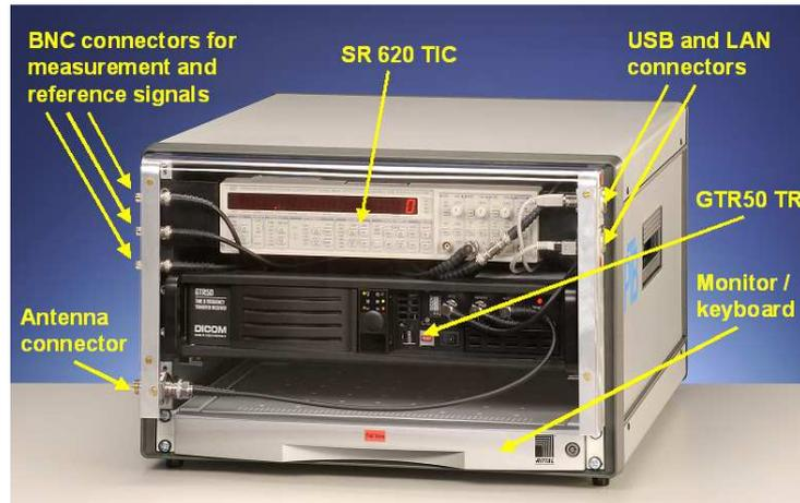
Figure 2. PTB's calibration set-up.
