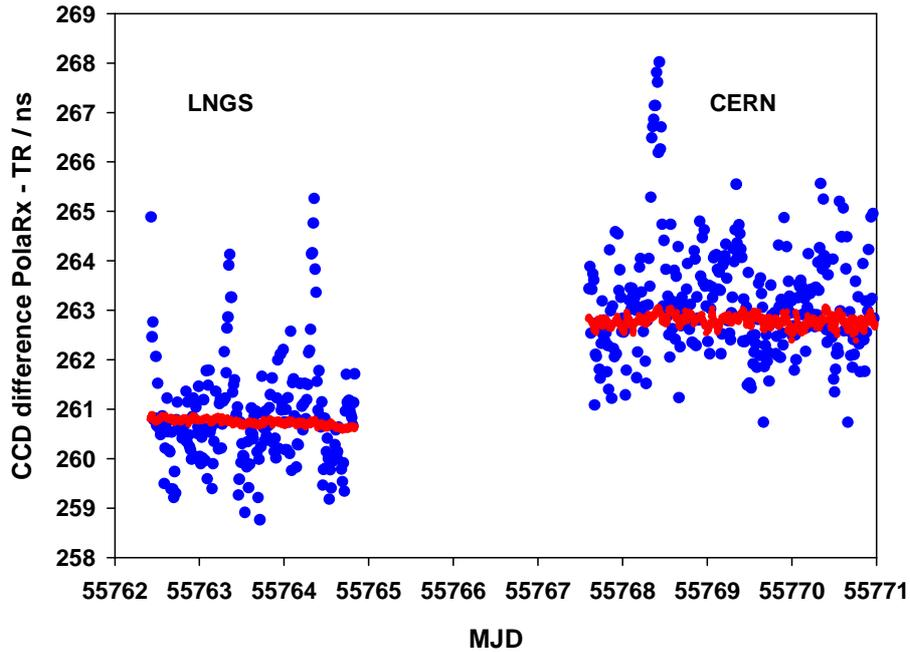
Figure 3. CCD results (blue: P3, red: PPP) at LNGS and CERN. The measurement period (x-axis) is given as Modified Julian Day
